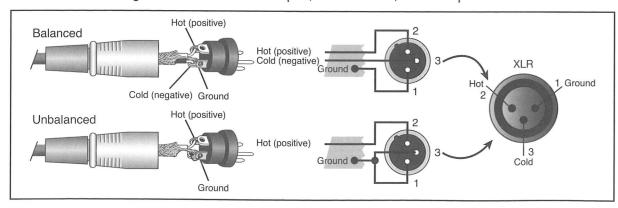
Turn PHANTOM switch OFF if using the unbalanced cable.
